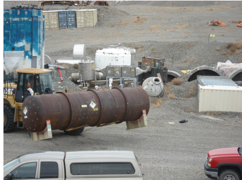
Disposal of one of the MFC sodium tanks following treatment of residual sodium
